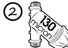
Add sufficient 130micron filters
